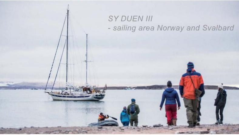
Year Built 1987 Length 22 m / 72 ft Sail Area 165 m² / 1,770.00 ft² Mast Height 20 m / 65 ft Main Engine Perkins Sabre 215 HP Cruising Speed 8 knots
